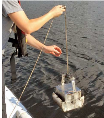
Open water samples were collected by using an Ekman grab
